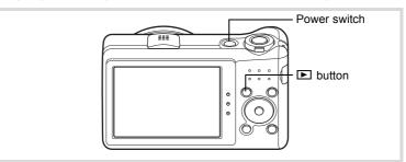
Press the power switch while holding down the button.
